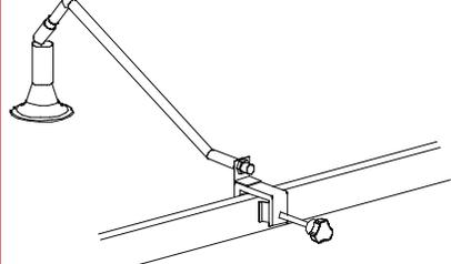
Attach Light to Horizontal Extrusion and secure clamp.
