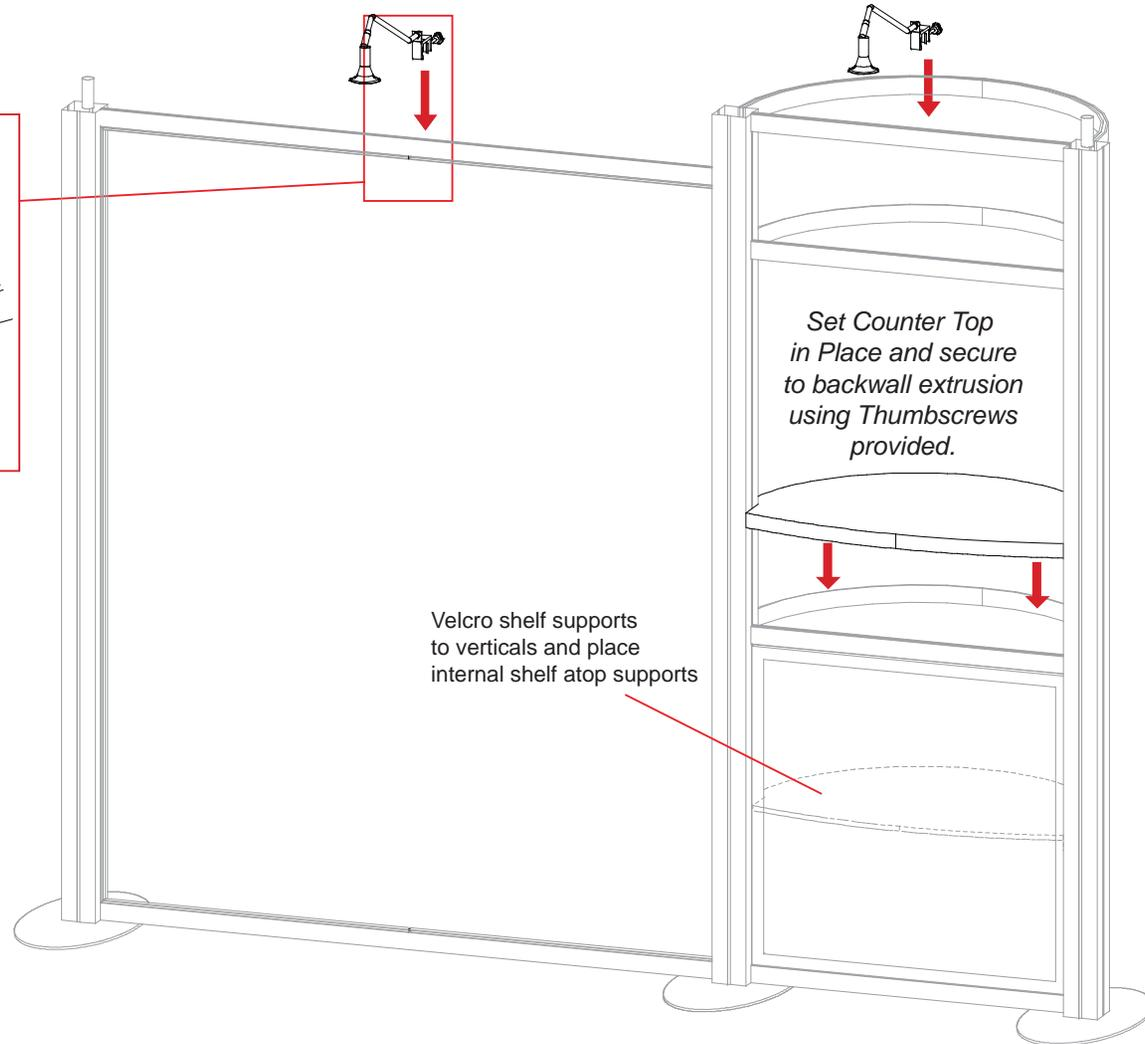
Set Counter Top in Place and secure to backwall extrusion using Thumbscrews provided.
