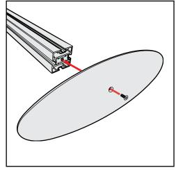
Base Plate & Extrusion Connection
