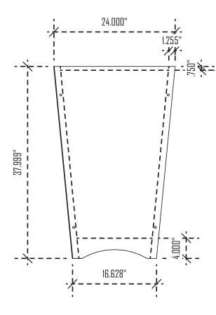
Internal dotted lines represent approximate inside dimensensions of side panels, floor, and counter edge.
