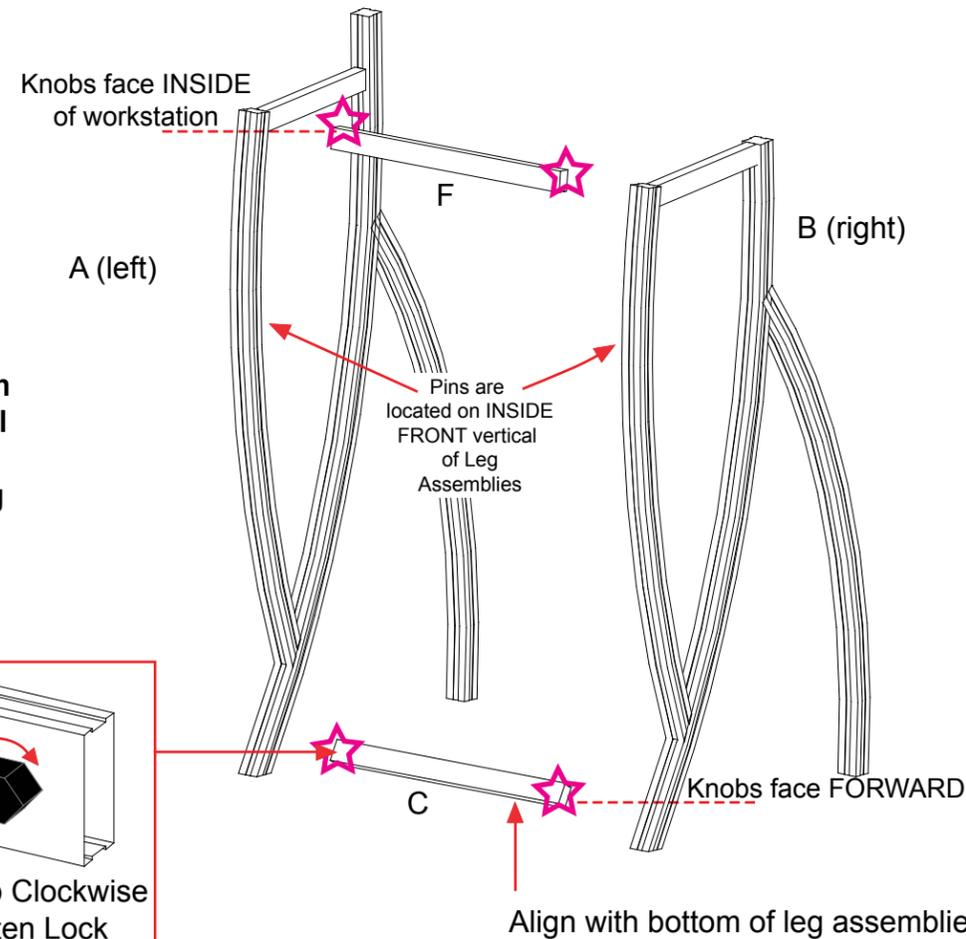
**NOTE: Make sure the lock is flush with extrusion before tightening. If lock will not fully engage, gently rock lock and extrusion back and forth while turning knob until lock fully opens.**
