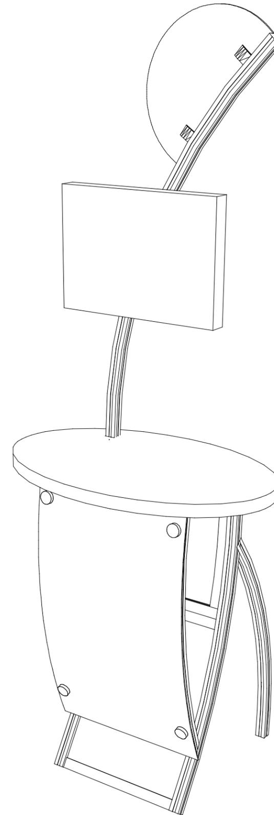
WHEN DISASSEMBLING ALUMINUM EXTRUSION, TIGHTEN ALL SETSCREWS AND LOCKS TO PREVENT LOSS DURING SHIPPING
